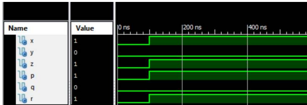
Figure 8: Output Waveform of the FRG Gate
